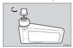
**2** Open the fuser oil bottle cover of the printer.
